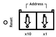
Before communication, you must assign a slave ID to the PROFIBUS slave, If you would like to assign an address between 0 - 99, you need to change the rotary switch to the desired address. If you would like to assign an address which is over 99, you must set it in the MGate utility.
