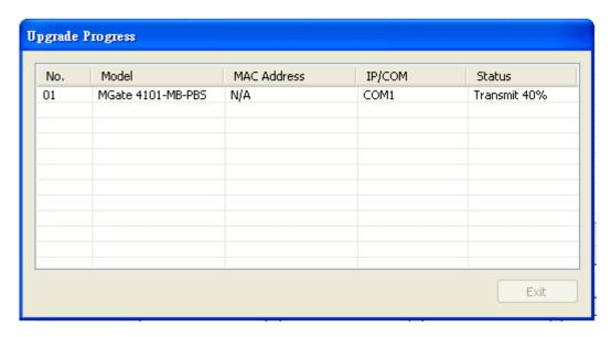
Once the firmware has been successfully written onto the unit, click **Exit** to close the Upgrade Firmware window. MGate Manager will automatically execute a Broadcast Search for all MGate units on the LAN and the recording COM port. Your MGate should reappear in the list of units.
