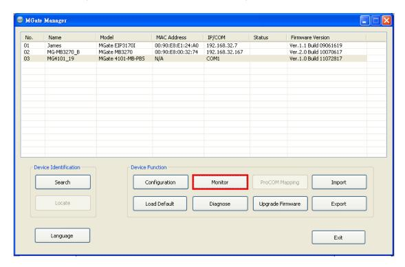
In the Traffic Monitor window, click **Start** to begin live monitoring of the data passing through the selected MGate 4101-MB-PBS unit.
