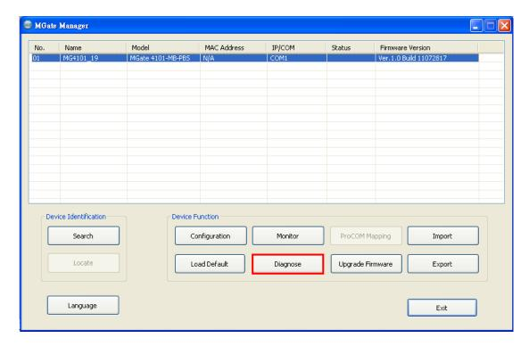
The dialog box will show the detailed of communication status of both Modbus and PROFIBUS, in addition it contains serial parameters.
