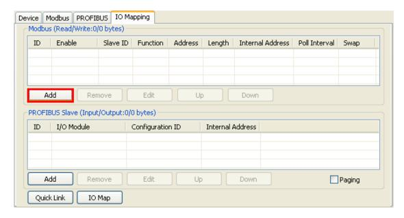
Each Modbus request includes Enable, Modbus slave ID, Function Code, Address, Length, Internal Address, Poll Interval, Swap. Please refer to datasheets or manuals of Modbus slave devices to fill out these fields.
