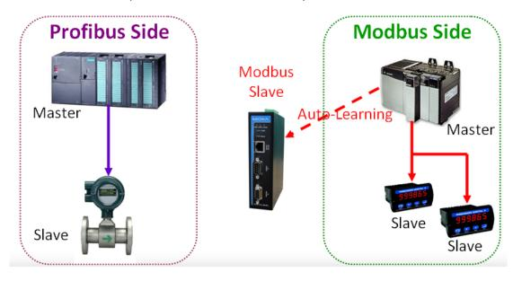
After some time, MGate 4101-MB-PBS will fully learn the requests from the Modbus master. Through this QuickLink process, the MGate 4101-MB-PBS can replace the legacy Modbus master. Moreover, the MGate 4101-MB-PBS can respond to all of the Modbus slaves correctly.
